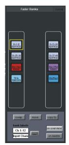
To swap the locations of two fader banks, touch one bank button so that it is highlighted in yellow, touch **swap** (located below the left fader bank's) and touch the other bank button.
