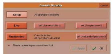
User passwords can be defined for the Live and Unattended modes. To set a password, press the Set Password button. Enter the old password, then enter the new password twice. By default, the passwords are blank.
