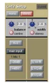
Stereo channels also have an **m-s** button, located above the input routing button, which switches in a decode function for replaying M-S signals as a normal stereo pair. There are three further buttons in this panel: L<>R swaps the channel's left and right outputs, L>L+R sends the left signal to both left and right busses, and R>L+R sends the right signal to both left and right busses.
