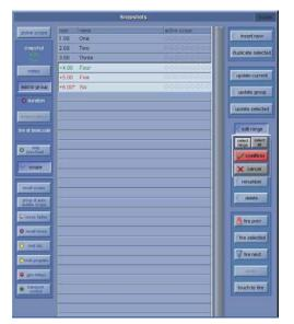
With the Edit button pressed, pressing the Snapshot buttons does not fire the snapshots, it only selects them for editing.
