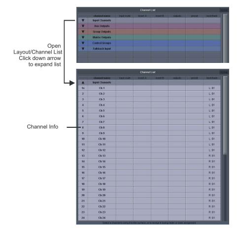
Primarily, the **Channel List** display is used for adjusting the bank assignments of the session's channels. This function employs the **COPY BANK FROM** LCD function mode, and is described in full in the Channel Types section of this manual.
