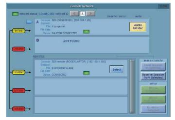
When running SD9 software on a PC the software will appear in a number of "floating" windows, each of which represent a console section. A screen touch on the console is simulated by a right click with the PC mouse. To switch between console sections use the small toolbar buttons that also appear on the screen marked Master/Left/Right/Overview.
