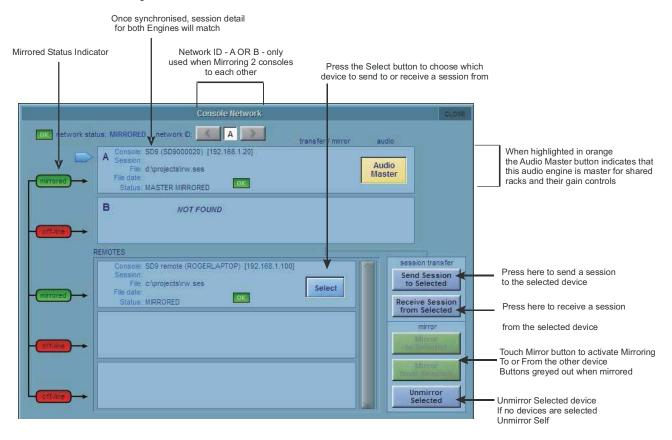
Note - The exact method of Mirroring is determined by a setting in the Options panel / Sessions tab - see below
