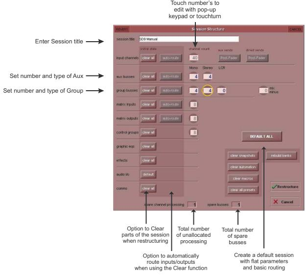
Note - Pressing the Default All button followed by the Restructure button will automatically configure a new session with the following setup where the first 32 rack inputs are routed to input channels 1-32 and the Master Buss is routed to Local outputs 1 & 2. All input channels will be routed to the Master Buss and the console headphones will be fed by the Master Buss when nothing else is soloed.
