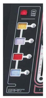
A 'bank' is a set of twelve faders, and a "section" contains up to four 'banks'. There are two sections of the desk, allowing up to 96 channels to be accessible on the worksurface.
