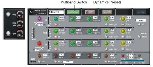
Up to 4 Channels can have their Dynamics (Compressor) modules switched into Multi-band mode
