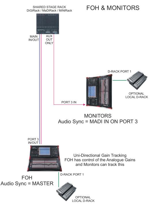
The recommended connection between the Monitor console and Stage Rack is a single MADI OUT from the Stage Rack's AUX MADI connected to the console's MADI 3 IN.
