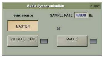
The SD9 will operates at a sample rate of 48000Hz (48kHz), and the current rate is indicated in the **SAMPLERATE** box at the top of the display.
