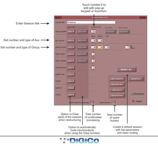
**Clear All Buttons**: When changing routing, you have the option of clearing any non-default routing or processing (EQ, dynamics etc) from the channels in the session. This is especially useful when restructuring an existing session to make a new session. The clear snapshots, clear automation and clear macro's perform similar operations.
