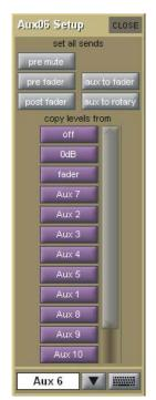
The grey set all sends buttons at the top of the Setup display affect the sends to that aux bus from all of the Input channels. The three buttons on the left, **pre mute**, **pre fader** and **post fader**, set the point in the channel from which the aux send is taken. The current send point is displayed next to the aux send level in the Input channels.
