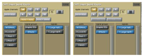
When routing to Internal FX using an auxiliary, the FX send is also configured according to the channel type (Mono or Stereo) but a Mono auxiliary can be set to provide a stereo FX output by pressing the **Mono>Stereo** button and rerouting.
